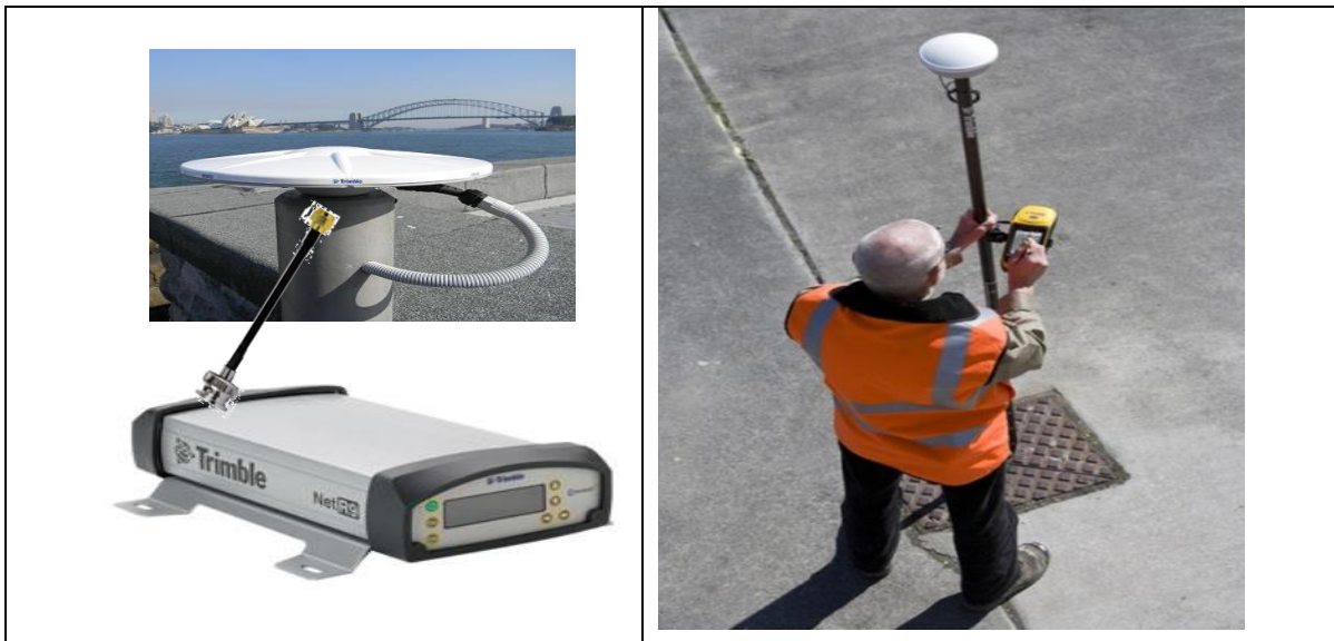
Fig-2 Reference Station and Rover Setup
