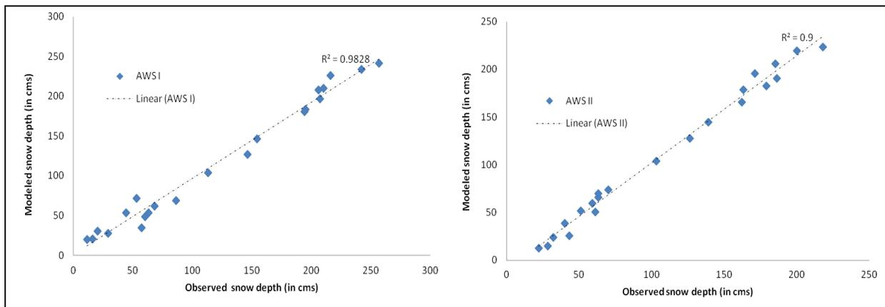
**Figure 3: Comparison of modeled and observed snow depth using AWS data**
