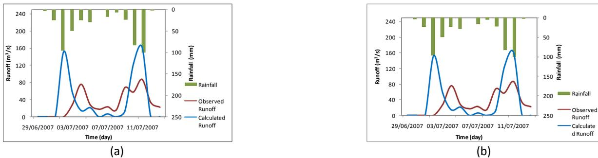
**Fig:6-Observed versus Predicted Runoff for Event-1 using (a) LANDSAT and (b) LISS-III.**
