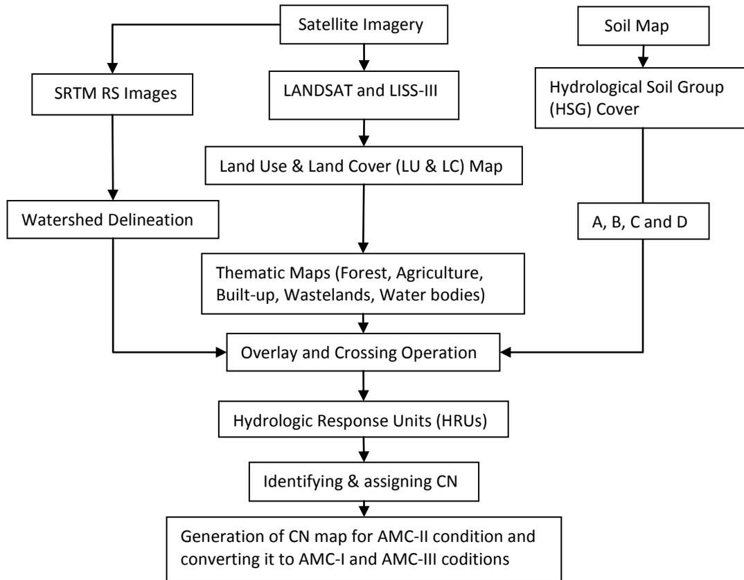
Fig:1- Flowchart Showing the Process of CN Generation
