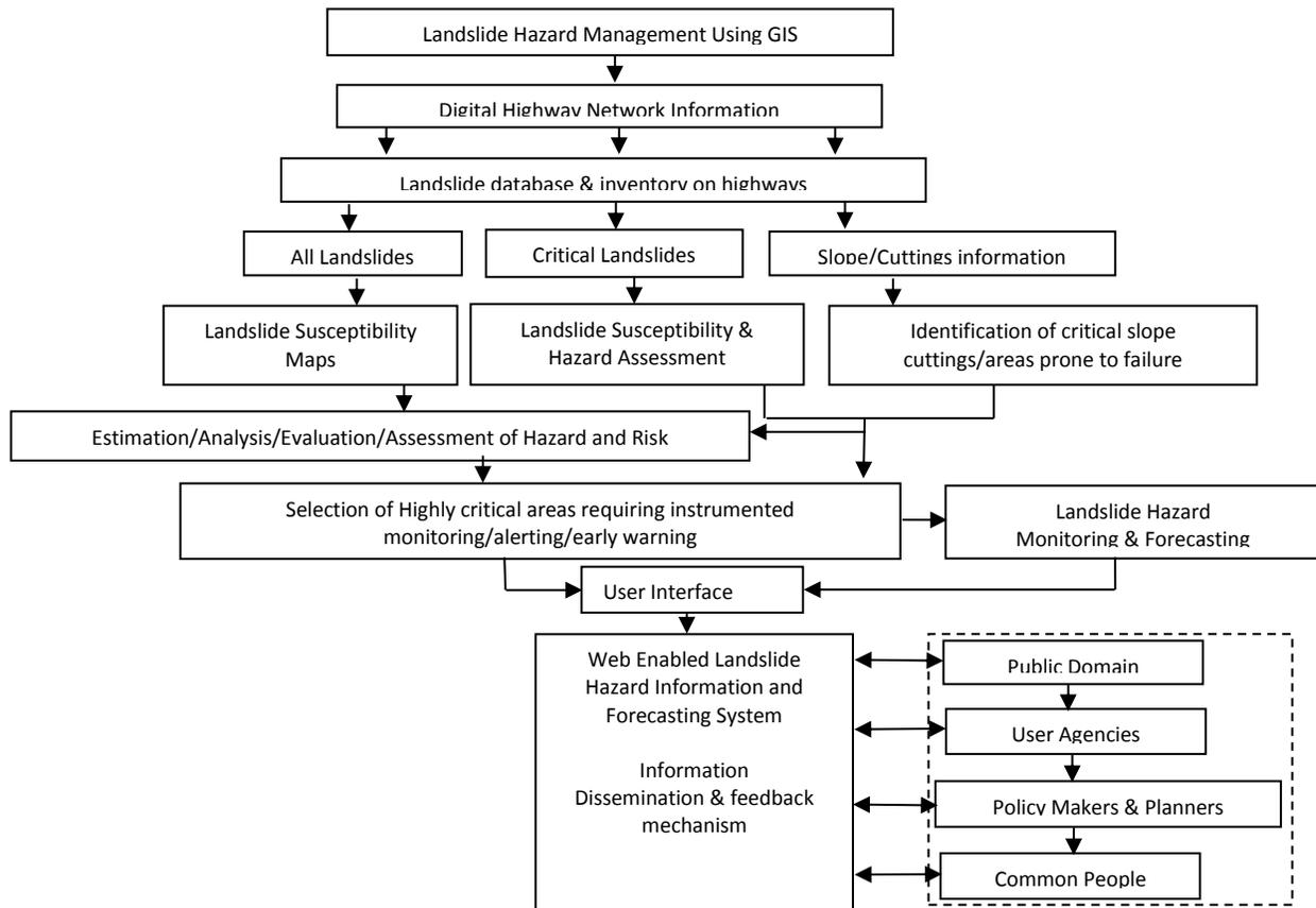
Fig 2 Landslide Hazard Management Plan Using GIS Application
