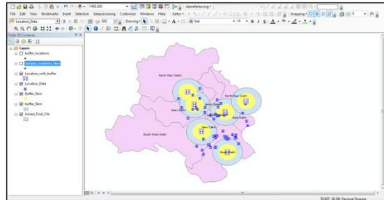
**Fig: 3- Buffer Analysis using ArcToolbox (ArcGIS)**
