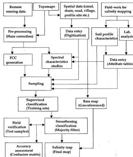
Figure 1 A Flow chart for salinity mapping using digital image analysis and GIS
