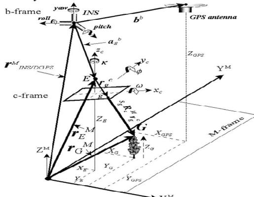
Where  $x_g^c$  and  $y_g^c$  are image coordinates of point g and  $x_{pp}^c$  and  $y_{pp}^c$  are offset points; k is a scale factor accounting for the nonsquareness of the CCD pixels; f is the calibrated focal length of the lens in use.
