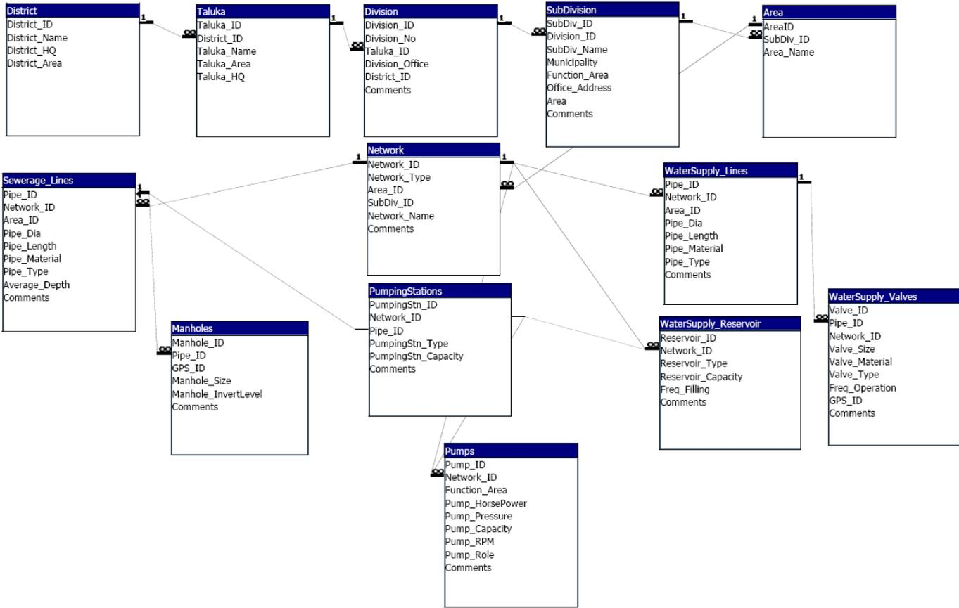
**Fig:3 – Data Structure for Asset Management System**
