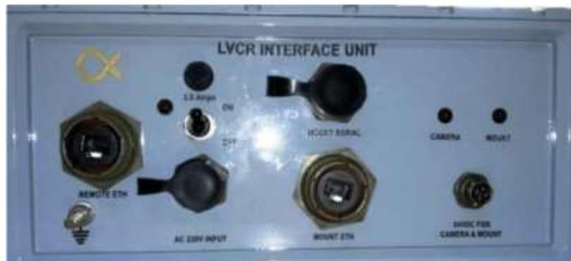
**Fig: 4 – Interface box to integrate the hardware with software**
