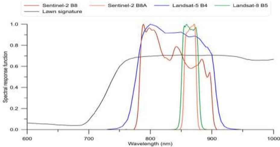
Fig: 1 Spectral response of Multispectral Instruments (MSI) onboard sentinel-2 [7], Operational Land Imager (OLI) onboard Landsat-8 [8], and Thematic Mapper 5 (TM5)
