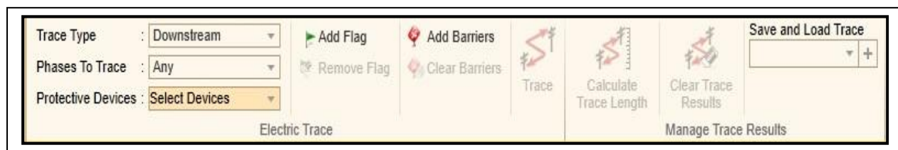
Fig: 3 – Tool bar developed for Electrical Tracing
