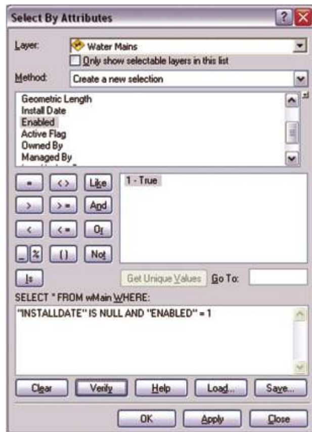
This sample Select by Attributes query has been configured to find water main features that are enabled and have a null value for the installation date.
