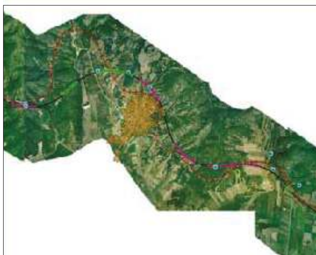
GIS can be used to develop complex, multicriteria models to help define an optimal transportation alignment, accounting for soils, slope, and other environmental constraints.
