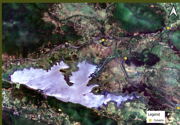
Culvert Location Identified using Super Resolution (SR3) tool in ArcGIS Pro
