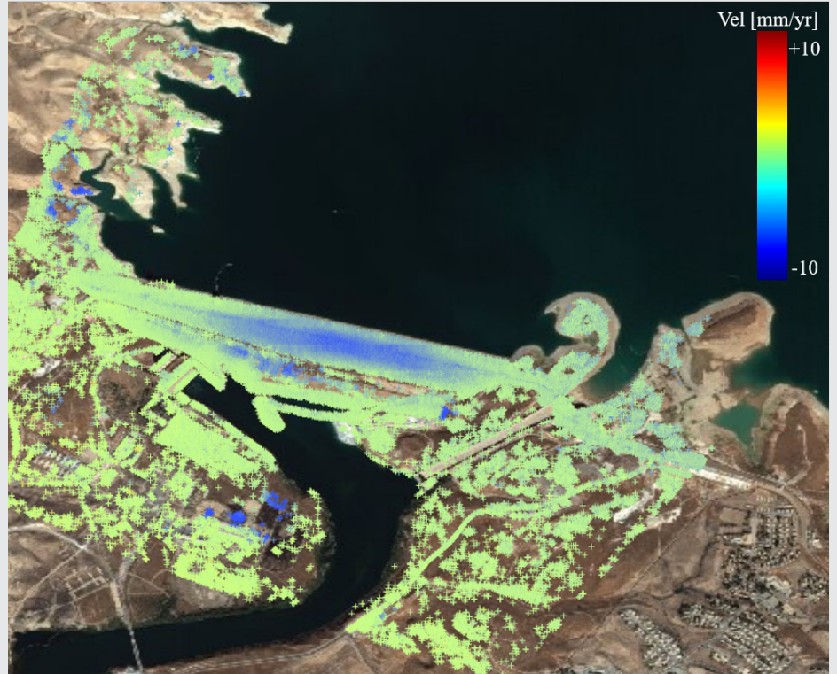
This image depicts the average displacement rate (color scale between -10 and +10 mm/year) at the Mosul Dam in Iraq. The source image is COSMO-SkyMed, processed using ENVI SARscape by sarmap SA.
