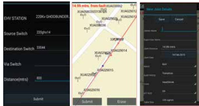
Fig 3: Fault Locator App on Mobile
