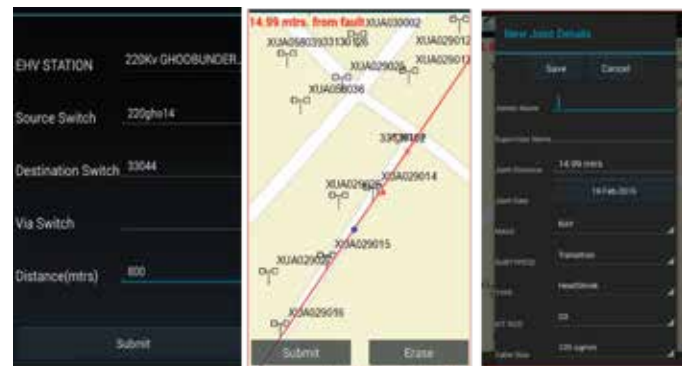
Fig 3: Fault Locator App on Mobile
